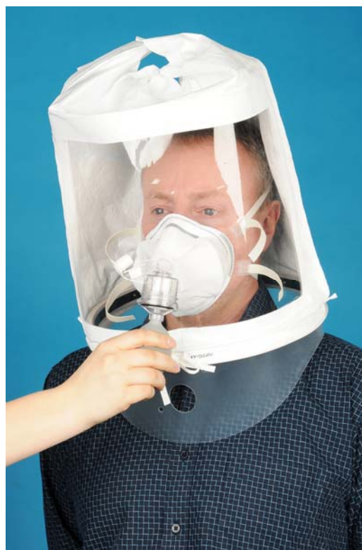
Fig. 7 Example of a qualitative fit test method
