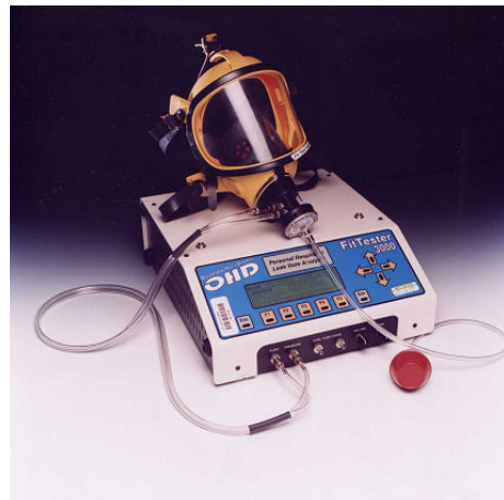
Fig. 10 Controlled negative pressure fit testing device
